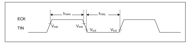
• Trigger input timing
